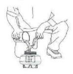
4. Attach the canister to the gun, plug in the cord.
