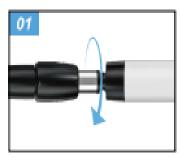
The rod with the threaded end is rotated and tightened with the machine head.
